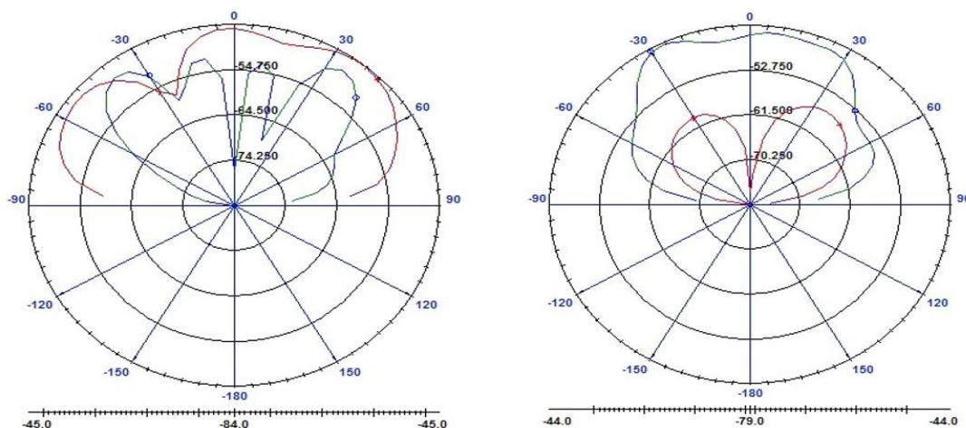
*Figure 5. Polar radiation pattern of array antenna without scan in E-theta and E-phi*
