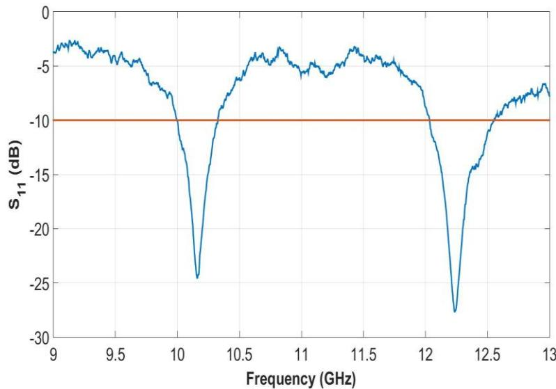
Figure 10. Return loss of phase array antenna with scan implemented
