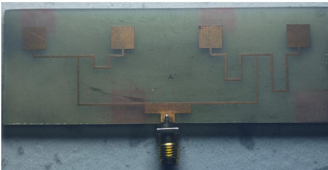
Figure 4. Phase Array Antenna
