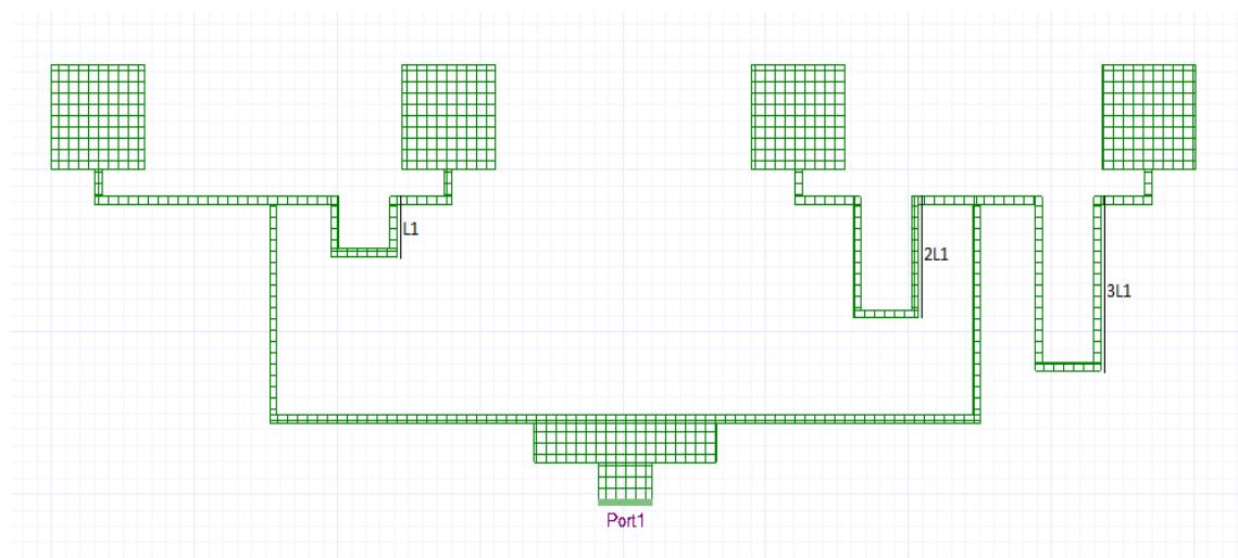
Figure 3. The final design of proposed antenna
