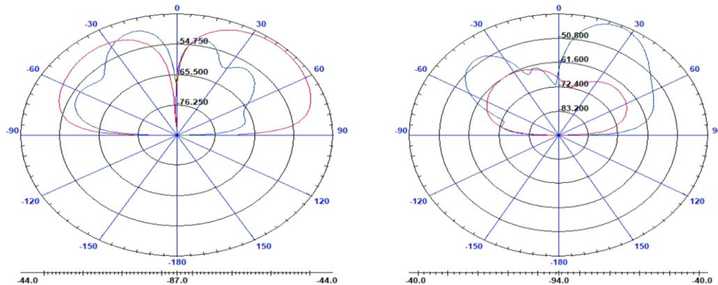
*Figure 6. Polar radiation pattern of array antenna with scan in E-theta and E-phi at 10.17 GHz*
