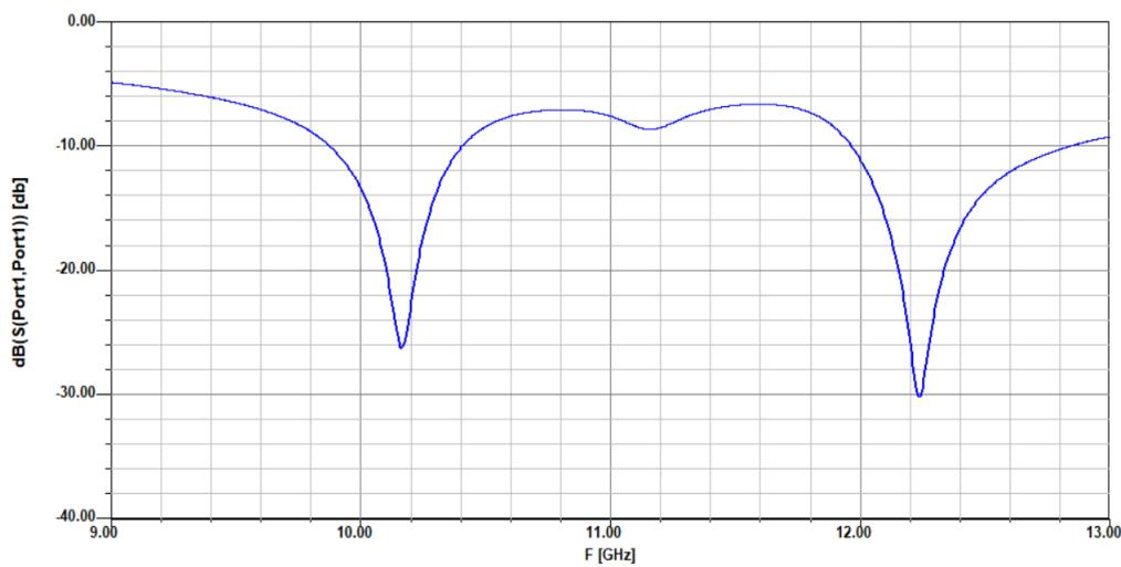
Figure 9. Return loss of phase array antenna with scan
