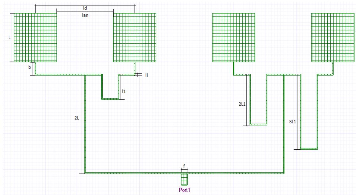
Figure 2. The geometry and parameters of proposed antenna
