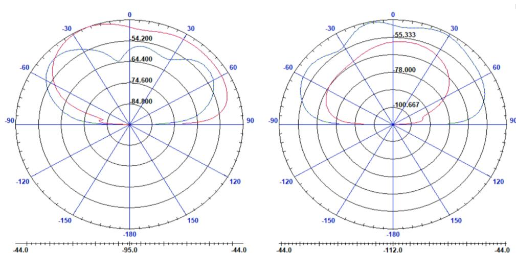
Figure 7. Polar radiation pattern of array antenna with scan in E-theta and E-phi at 12.34 GHz
